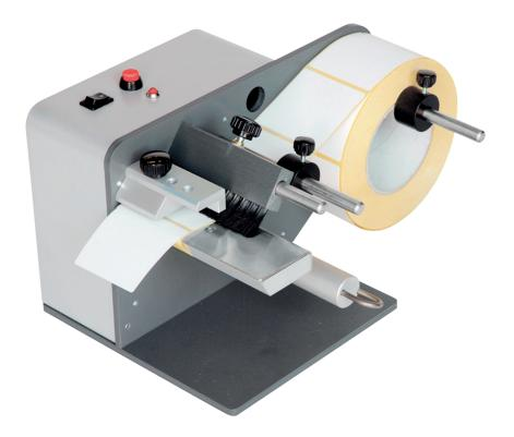
Automatic label dispenser suitable for not transparent self-adhesive label. The labels are read by 2 sensors that could identify the difference in transparency existing between the labels. After the removal of a label from the paper support, teh next label will stick out automatically.
